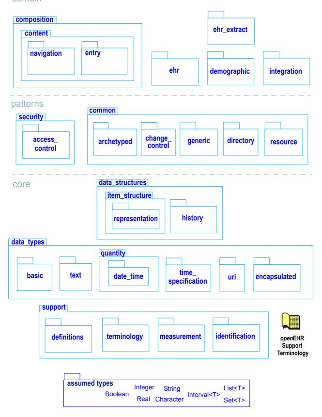
FIGURE 10 Structure of org.openehr.rm package
