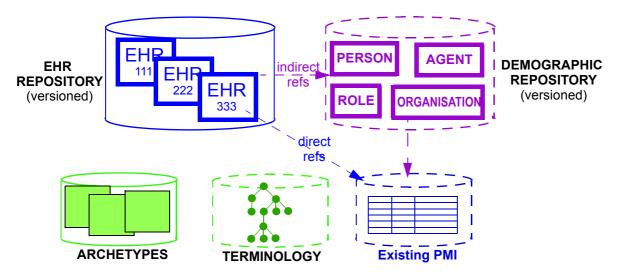
FIGURE 13 Minimal openEHR EHR System
