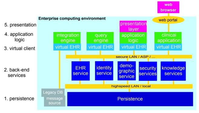
FIGURE 37 Basic Enterprise EHR System Architecture
