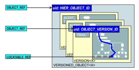
FIGURE 29 How to reference various levels of object
