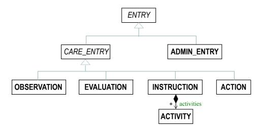
FIGURE 16 The openEHR Entry model (in EHR IM)
