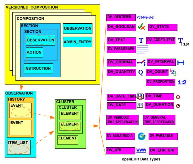
FIGURE 15 Elements of an openEHR Composition
