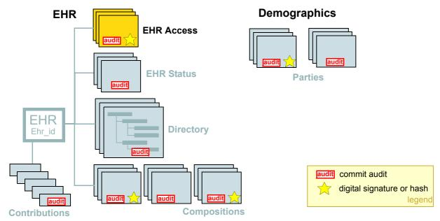
FIGURE 21 Security Features of the openEHR EHR
