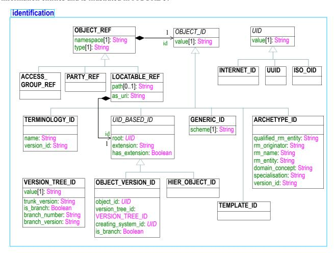
FIGURE 5 rm.support.identification Package
